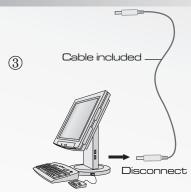
Disconnect the other end of the USB cable from the USB port on the computer.
